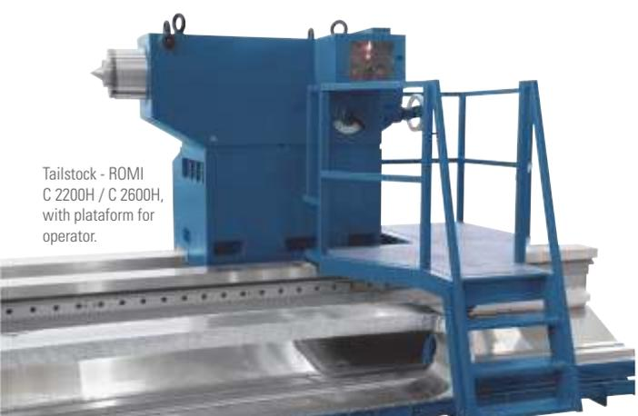
Tailstock - ROMI C 2200H / C 2600H, with platform for operator.
