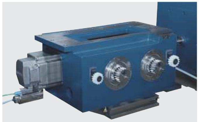
Pre-loaded Double pinion system (Redex)
