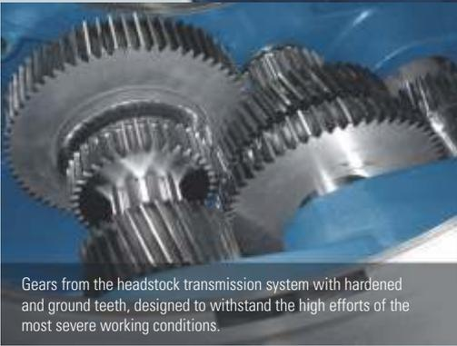
Gears from the headstock transmission system with hardened and ground teeth, designed to withstand the high efforts of the most severe working conditions.
