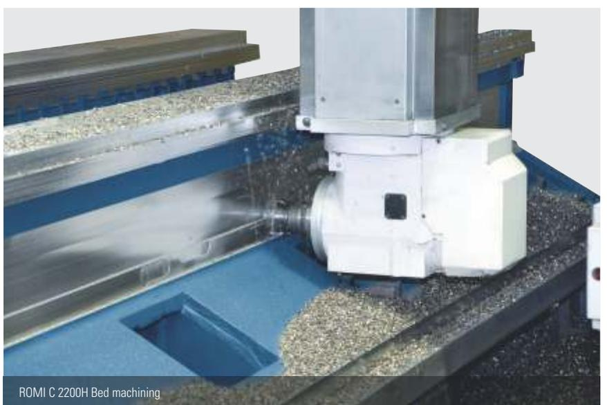
Cast iron robust housing, internally ribbed to absorb high efforts of heavy machining operations.
