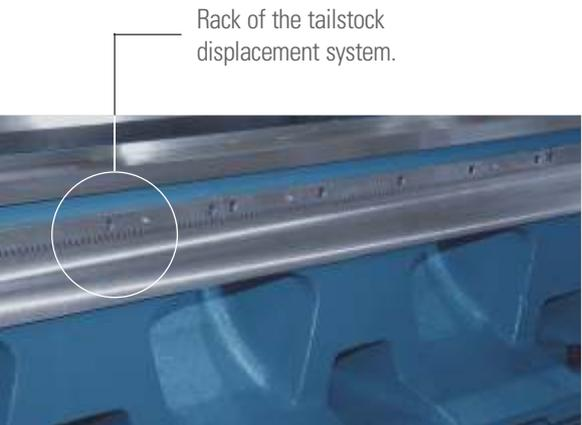
Rack of the tailstock displacement system.
