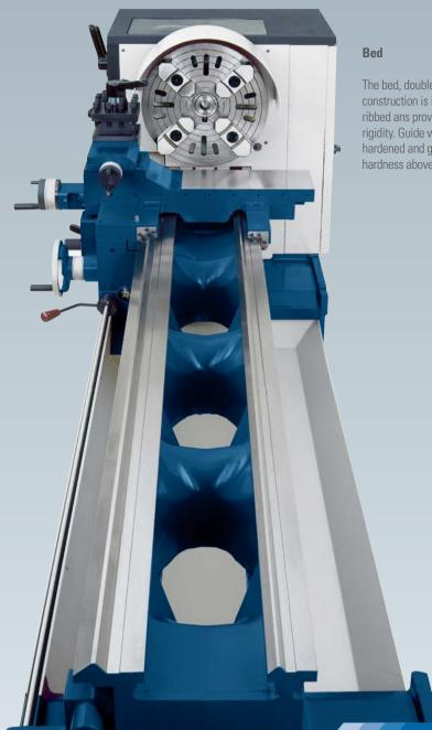
The bed, double wall, construction is internally ribbed ans provides excellent rigidity. Guide ways are hardened and ground with hardness above 450 Brinell.
